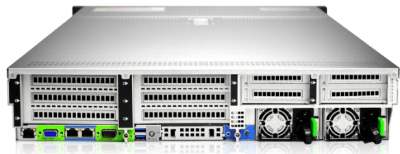
Rear View of 10 PCIe Slots
